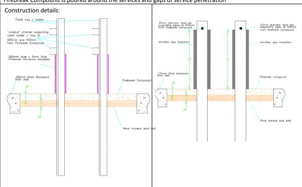
Firebreak Compound is poured around the services and gaps of service penetration
